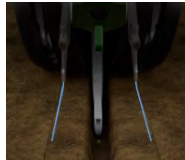
Figure 2. Conceal Dual Placement 3” from Seed Trench, 1.5” in Depth
