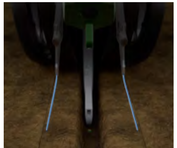
Figure 2. Conceal Dual Placement 3” from Seed Trench
