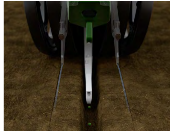
Figure 2. Conceal Dual band fertilizer
