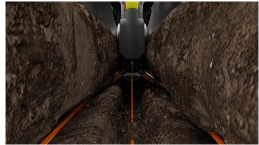
Figures 2-3: FurrowJet® Dual-Band Wings Fracturing Sidewalls
