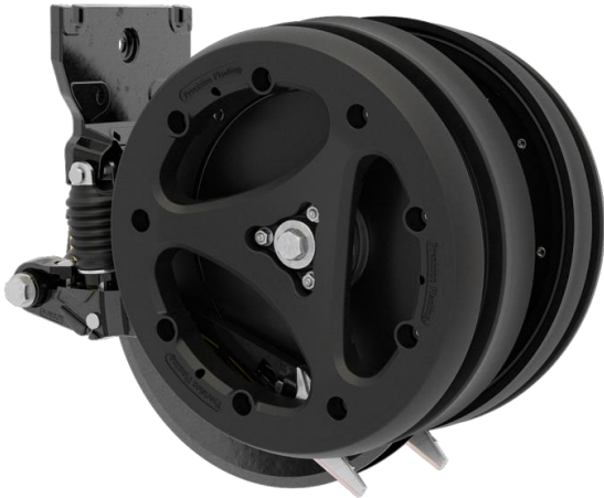
Figure 1. Conceal® System Knife Design within Gauge Wheel
