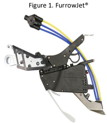
Figure 2: FurrowJet® Dual-Band Wings Fracturing Side-Walls
