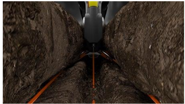
Figure 2: FurrowJet® Dual-Band Wings Fracturing Side-Walls
