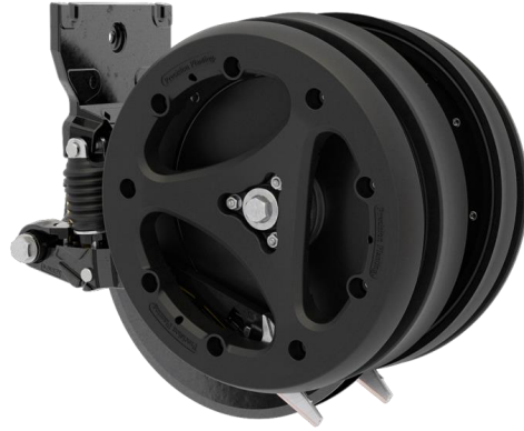
Figure 3. Conceal® 3" away, 1.5" deep from the seed trench
